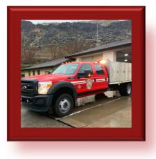
**Brush Trucks** are designed to fight wildfires. They have higher clearance to go offroad, and they carry tools such as picks, shovels, axes, and chainsaws. They also carry water and fire retardants suitable for stopping the spread of wildfires.
