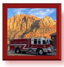
**Engines** carry water and firefighting equipment (such as axes, hoses, and nozzles). They also carry life-saving equipment and extrication tools.
