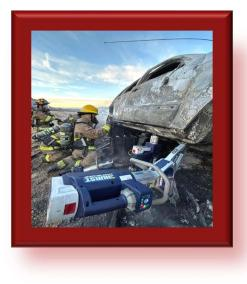
Jaws of Life are used to cut, spread, or push virtually any material to create openings for, and access to, patients.
