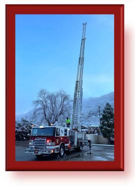
**Ladder Trucks** are used for hard-to-reach rescues, including those trapped on upper floors. They also provide safer and more efficient ways of fighting fires from above. Life-saving equipment is also on the trucks, much like the equipment on Engines.
